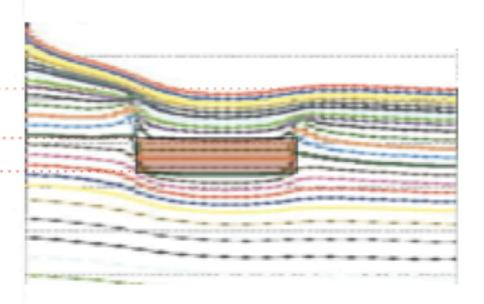
Left: A model of a flat lying conductor in a variably resistive background.
